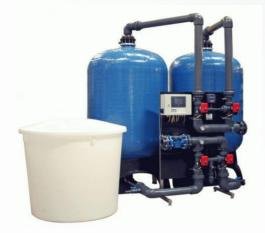
Our water softening systems prevent scale formation by removing calcium and magnesium ions from the water. Equipped with resin tanks, these systems are available in capacities from 0.005 m3/h to 100 m3/h and are designed to reduce costs and extend the life of equipment in plants using hard water.
