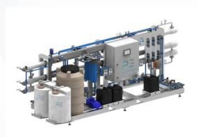
Reverse osmosis systems are a system in which dissolved organic and inorganic substances are removed from water by passing water through membranes at high pressure. With capacities ranging from 0.005 m3/hour to 50 m3/hour, these systems are ideal for drinking water production from seawater and industrial plants that need ultra-pure water. The efficiency of the system depends on the quality of the membranes, pumps and automation systems used.
